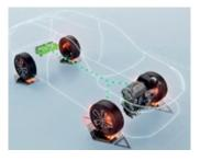
Regenerative braking uses the energy generated by the electric motor when braking to recharge the main drive battery
