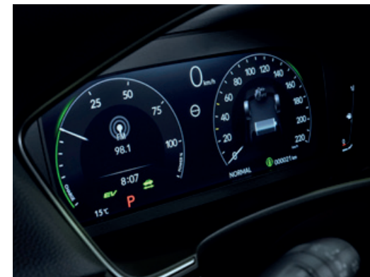
Above: as standard, Sport models come with a 7" dash display, above, while Advance has a 10.2" high definition TFT screen
