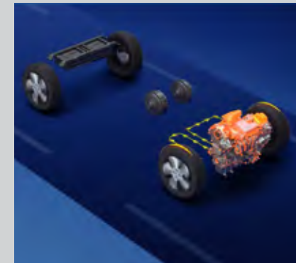
Engine Drive A 97PS petrol engine drives through the e-CVT automatic transmission, for spirited performance and optimum fuel economy
